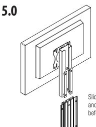
Slide LCD mount unto track into desired position and tighten all bolts. Ensure the mount is secure before installing any technology.
