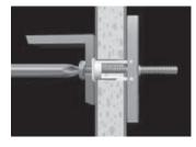
• Gently hand engage at least one thread of bolt with channel before using screw gun to avoid cross threading the bolt.
