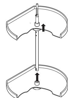
**Step 7** Starting with the top shelf, temporarily raise the shelf to the top of the pole above the last set of shelf positioning holes and push a bearing pin (E) through the pole at desired location. Lower shelf onto pin. Repeat this process with the remaining shelves.
