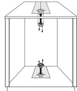
**Step 2** Fasten each of the Universal Mounting Plates (C) with (2) #8 x 1/2" Screws (F) using the slots so that future adjustment can be made, if necessary.
